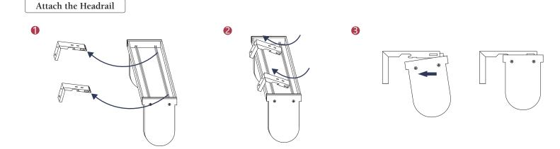
Align the headrail with the brackets and push it into place until it clicks securely.
