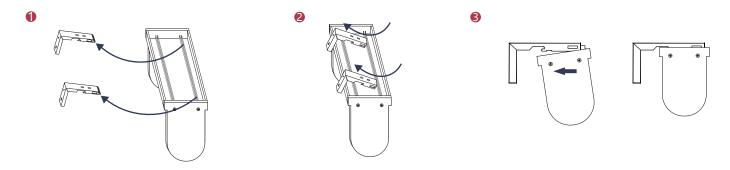
Align the headrail with the brackets and push it into place until it clicks securely.
